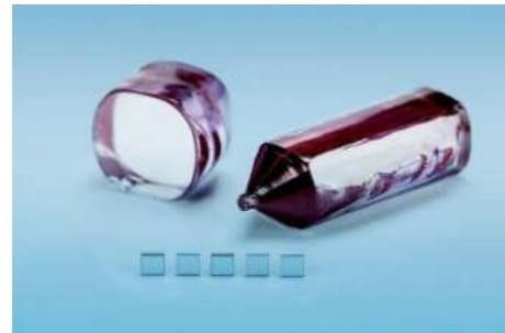
CASIX applies Czochralski (CZ) crystal growth technology to grow high-grade Nd: YVO<sub>4</sub> crystals. With strict control of materials and the growth process, our Nd: YVO<sub>4</sub> crystals feature low-lasing wavelength absorption and high conversion efficiency. CASIX offers Nd: YVO<sub>4</sub> crystal boules with doping rates from 0.1atm% to 4.0atm% and crystal components in various sizes and coatings.
